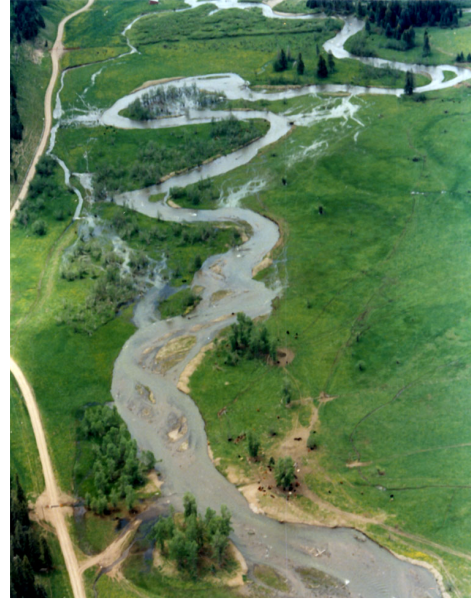
Figure 3. Stream channel adjustment from C4 to D4 stream type showing aggradation, lateral accretion, enlargement and potential avulsion, Weminuche Creek, Colorado, 1986 (photo by D. Rosgen).
